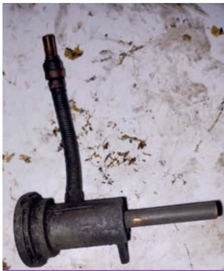
1. The waxstat jet removed from the carburettor.
