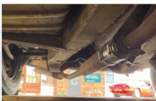
OLD-SCHOOL TIN CAN EXHAUST REPAIR
