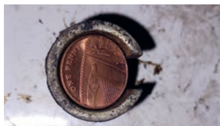
4. A penny is used to replace the wax module.
