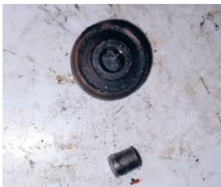
3. The waxstat thermostat and the button.
